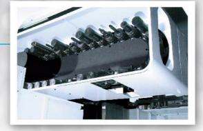
The 32-station chain-type tool magazine is driven by an electric motor (KMC-1500V)
