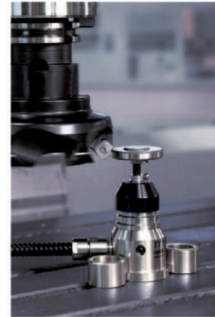
AUTOMATIC TOOL LENGTH MEASURING SYSTEM
